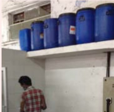
Chemicals stored at excessive height
